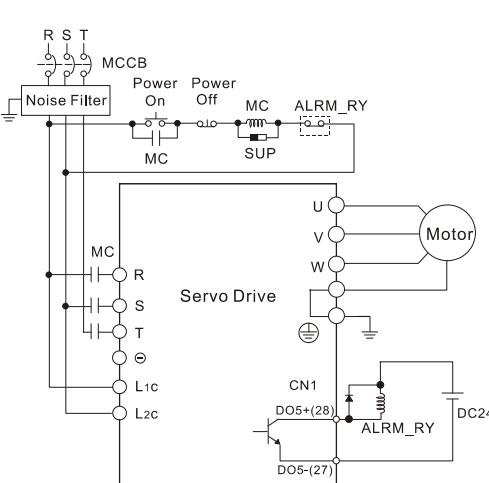
750W model (with built-in regenerative resistor but without cooling fan)
