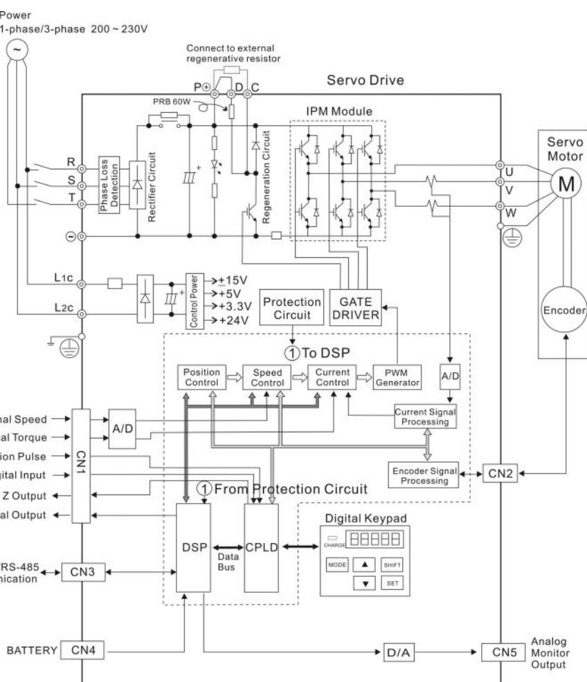
2kW~3kW models (with built-in regenerative resistor and cooling fan)
