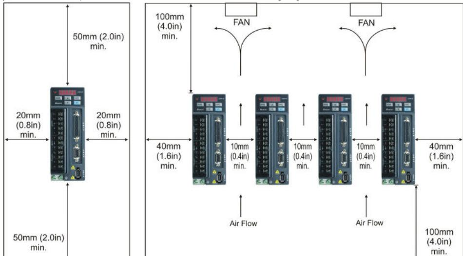
**NOTE** 1) The scale of the clearances does not match the dimensions as shown in the drawing above. In the event of any discrepancy between the clearances and the dimensions, the dimensions shall prevail.
